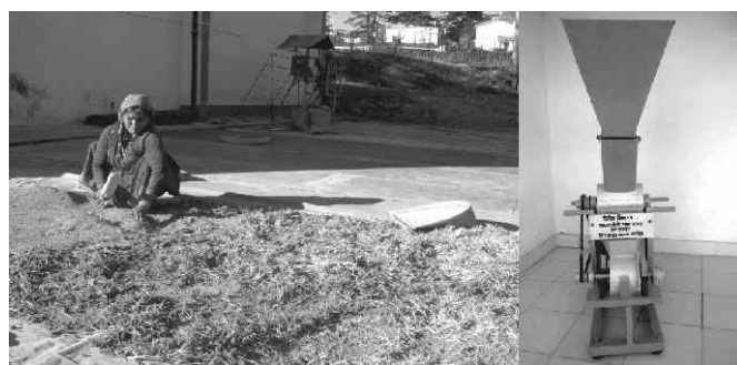
Fig.3: Threshing of finger millet through traditional practice and finger millet thresher cum pearler
