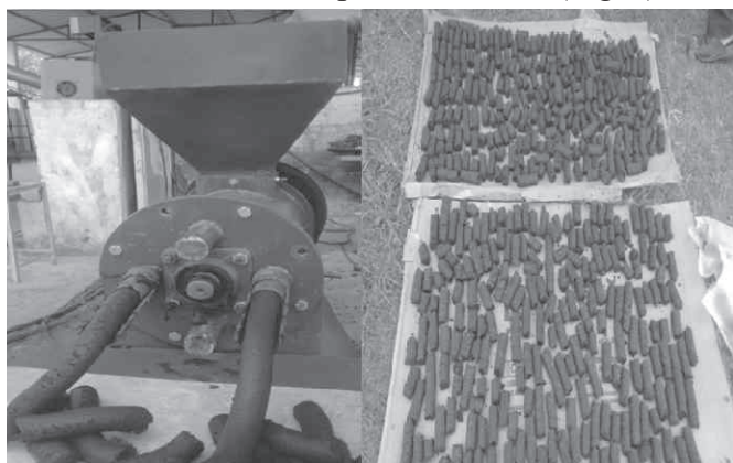
Fig.3. Crop residue briquetting machine and dried briquettes
