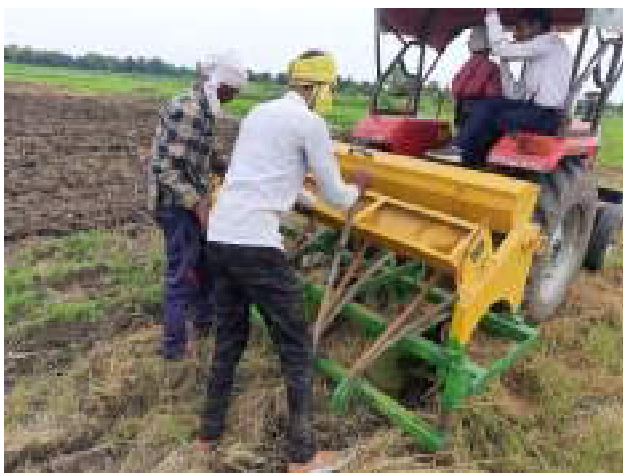
Fig: Use ferti cum seed drill machine. Sow in lines, apply fertilizer and conserve moisture with the zero-till ferti-drill.
