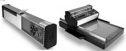
provided. Initially zero is set. When a leaf is placed in the conveyor belt it moves along with conveyor belt and when the leaf comes close to scanning camera, it reflects the image of leaf on the mirror and the reading is measured digitally. Area of leaf is expressed in cm<sup>2</sup>.
